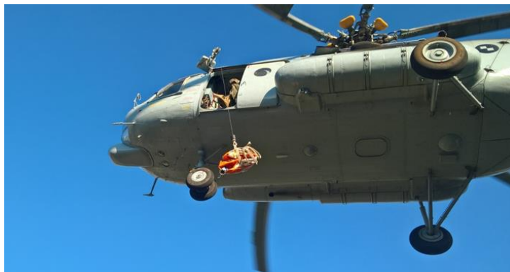
Hoisting a load using the LPG 150 winch
